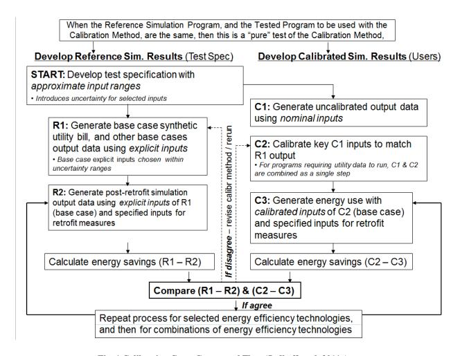
Fig. 1 Calibration Cases Conceptual Flow (Judkoff et al. 2011a)
