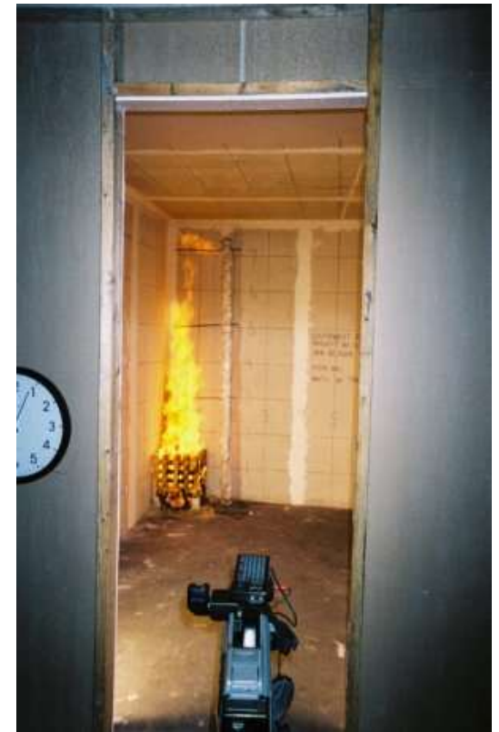
Figure 2. Room-corner fire test geometry.
