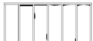
Grade II must be insulation installed with anomalies found to be between  $\frac{1}{2}$ % and 2% for all inspected walls, floors and ceilings of the building.
