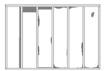
Grade III must be an insulation installation having between 2% and 5% anomalies found for all inspected walls, ceilings and floors of the building enclosure.
