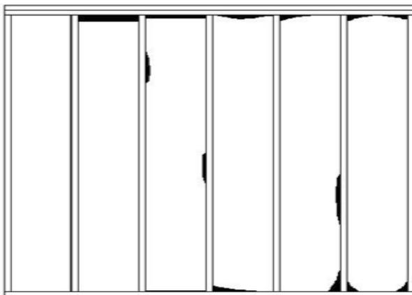
Grade II must be insulation installed with anomalies found to be between ½% and 2% for all inspected walls, floors and ceilings of the building.
