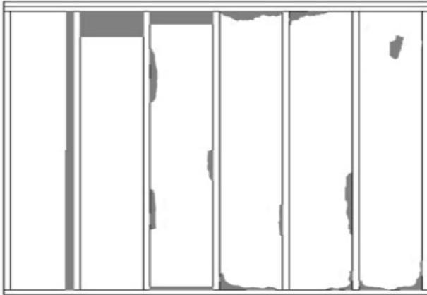
Grade III must be an insulation installation having between 2% and 5% anomalies found for all inspected walls, ceilings and floors of the building enclosure.
