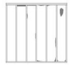
Compression or incomplete fill amounting to 2% or less, if the empty spaces are less than 30% of the intended fill thickness, are acceptable for "Grade I".
