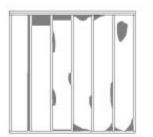
No more than 10% of surface area of insulation compressed or incomplete fill, by up to 30% (70% or more of intended thickness) is acceptable for "Grade II".
