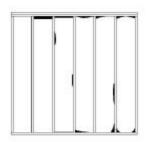
No more than 2% of surface area of insulation missing is acceptable for "Grade II"
