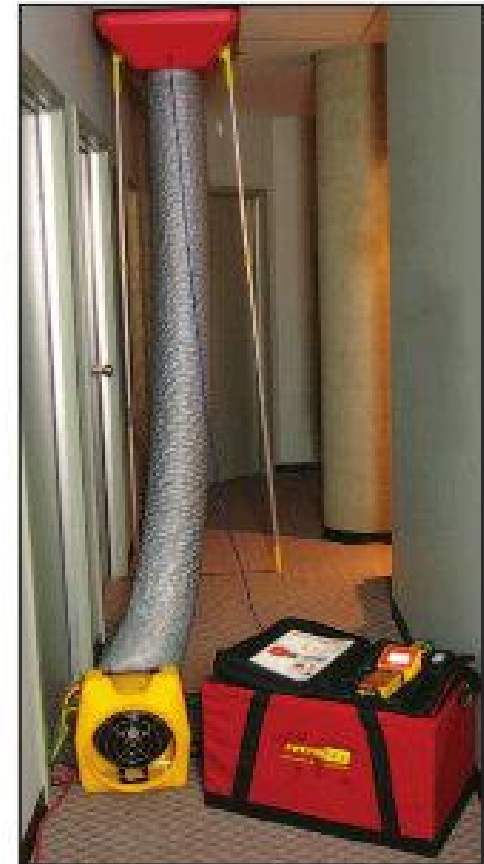
Pressure Pans for use as Powered Flow Hood #PP105
